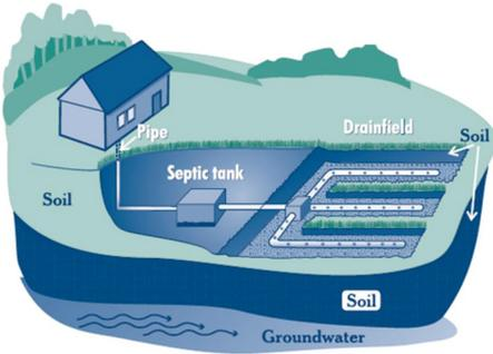
Water from the tank is pushed into the drainfield each time new wastewater enters the tank. Once in the drainfield, wastewater will percolate into the soil, which provides final treatment by removing harmful bacteria, viruses, and nutrients. Having appropriate soils is critical for successful wastewater treatment.
